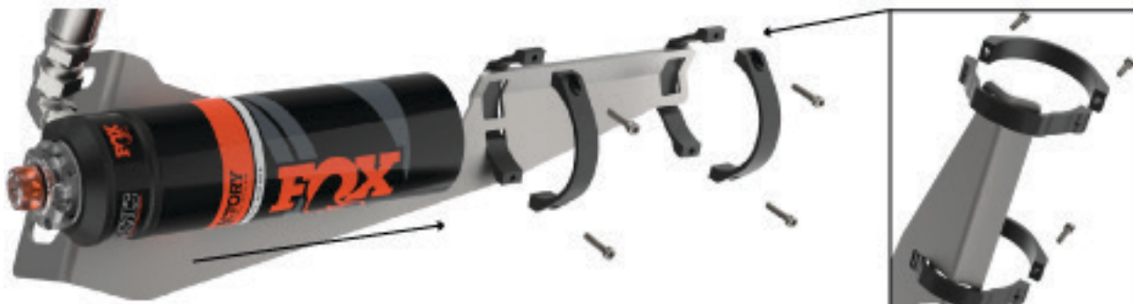
Fig. 10: Diagram of reservoir and bracket interface.
