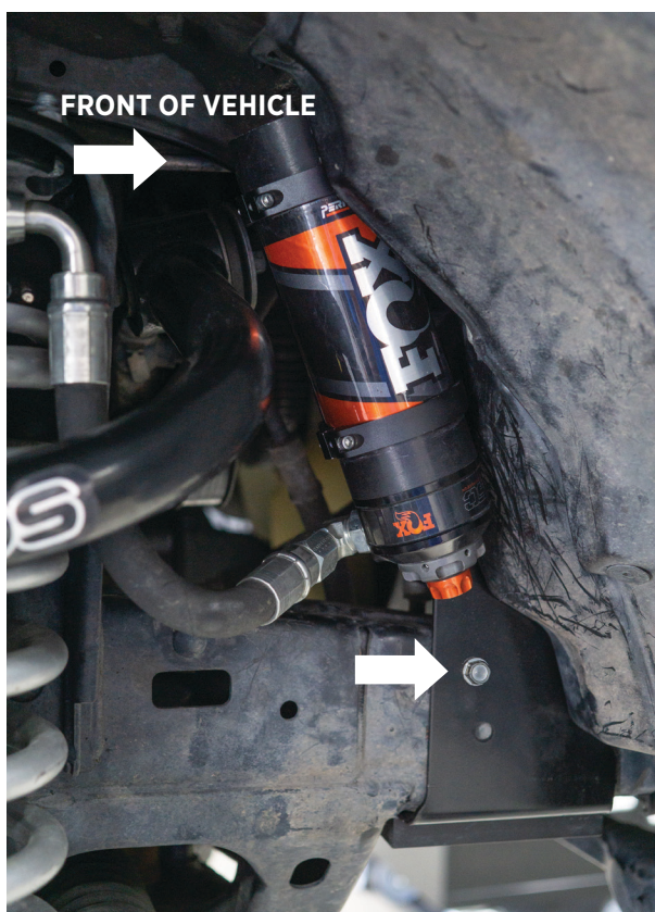
Fig. 13: Install the self tapping screw into the existing hole.
