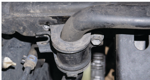
Fig. 11: Remove sway bar bracket.
