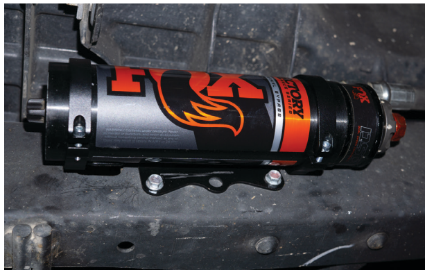
Fig. 24: Mount the reservoir to the bracket (passenger side shown).
