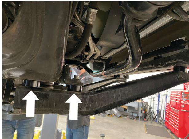
Fig. 16: Install the skid plate spacers
