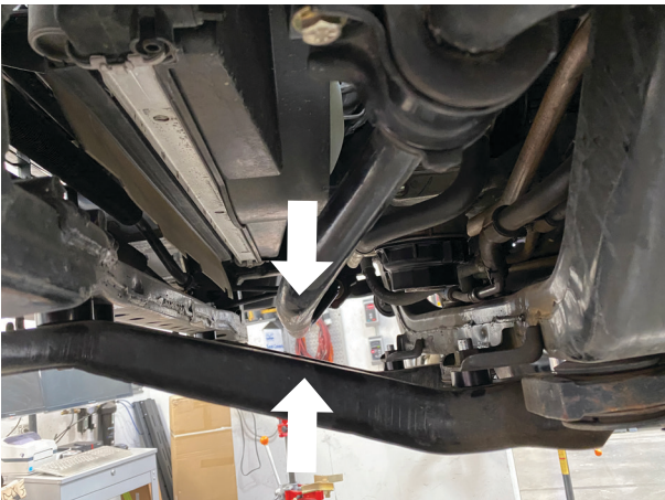
Fig. 15: Check clearance of the sway bar.
