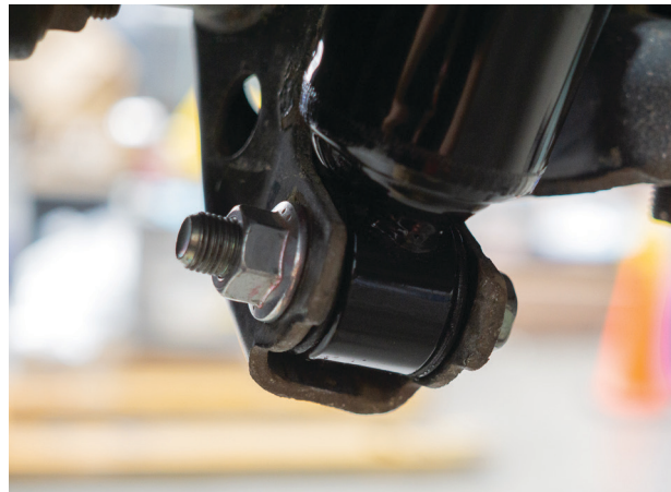
Fig. 20: Remove lower shock mount bolt.
