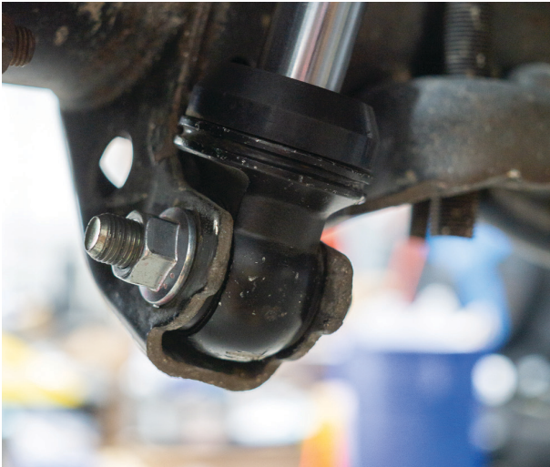
Fig. 22: Install the lower shock bolt (passenger side shown).
