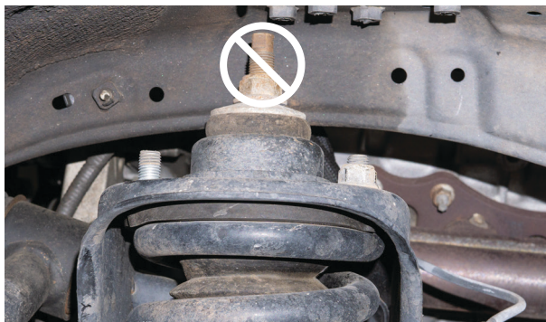
Fig. 4: Remove the three top hat nuts.
